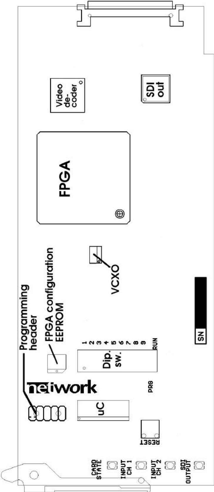
Figure 3: ADC-SDI simplified silkscreen (figure not to scale).
