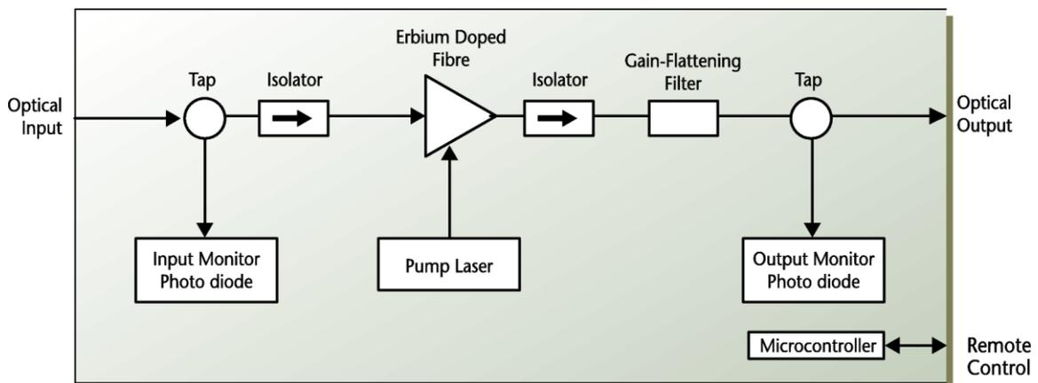
Figure 1: EDFA block diagram
