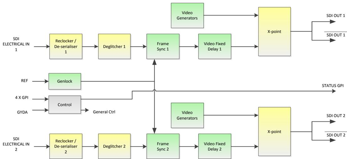
Figure 1: Simplified block diagram of the FRS-3G-DUAL card
