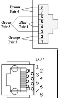
The diagram shows two views of the TP45 8-pin modular jack. The top view shows the wire pairs: Brown Pair 4 (pins 8, 7), Green Pair 3 (pins 6, 5), Blue Pair 1 (pins 4, 3), and Orange Pair 2 (pins 2, 1). The bottom view shows the pin header with pins numbered 1 through 8.
