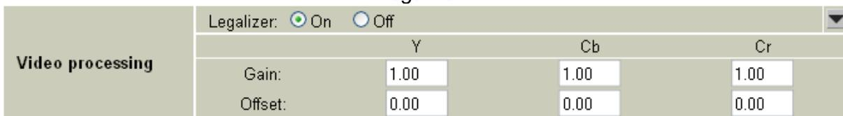
Figure 10: Multicon GYDA view of the video processing block
