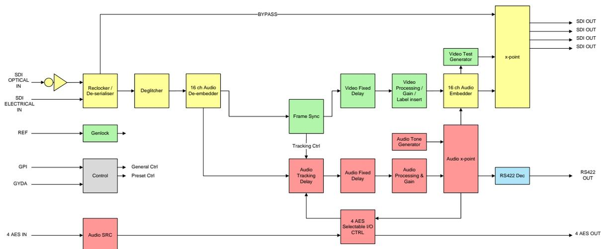
Figure 1: Simplified block diagram of the FRS-HD-XMUX4 card
