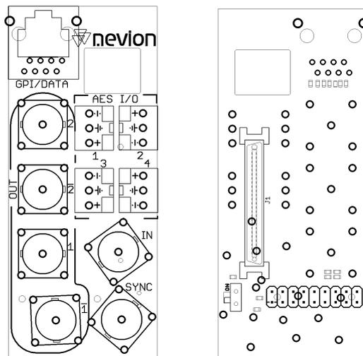
Figure 4: FRS-HD-XMUX4-C1 backplane
