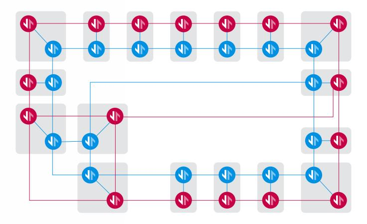
eMerge may also be used to build a WAN network on top of an optical infrastructure and offers full flexibility with regards to network topology (in combination with VideolPath).
