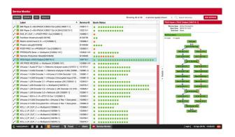
All monitoring information is also available on the REST API for integration with other systems. There are several examples of such integrations e.g. with the DataMiner monitoring system. In addition, the alarm information may be forwarded on SNMP to other northbound systems. Alarms are forwarded on a normalized format and enriched with service impact information.
