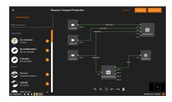
Within the Flow app, several pre-planned service definitions may be stored as templates and instantiated on demand (either immediately or scheduled). Activation of groups is available over the REST interface, which means that an external system can activate groups in a single operation.
